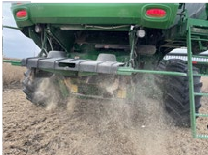
Above is the weed seed destructor that Jha used in his study. Photo provided by Prashant Jha, ISU.
